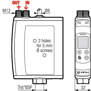
Mounting from side is the simplest to implement: Two Ø 5 mm through screws or bolts with large washers.
