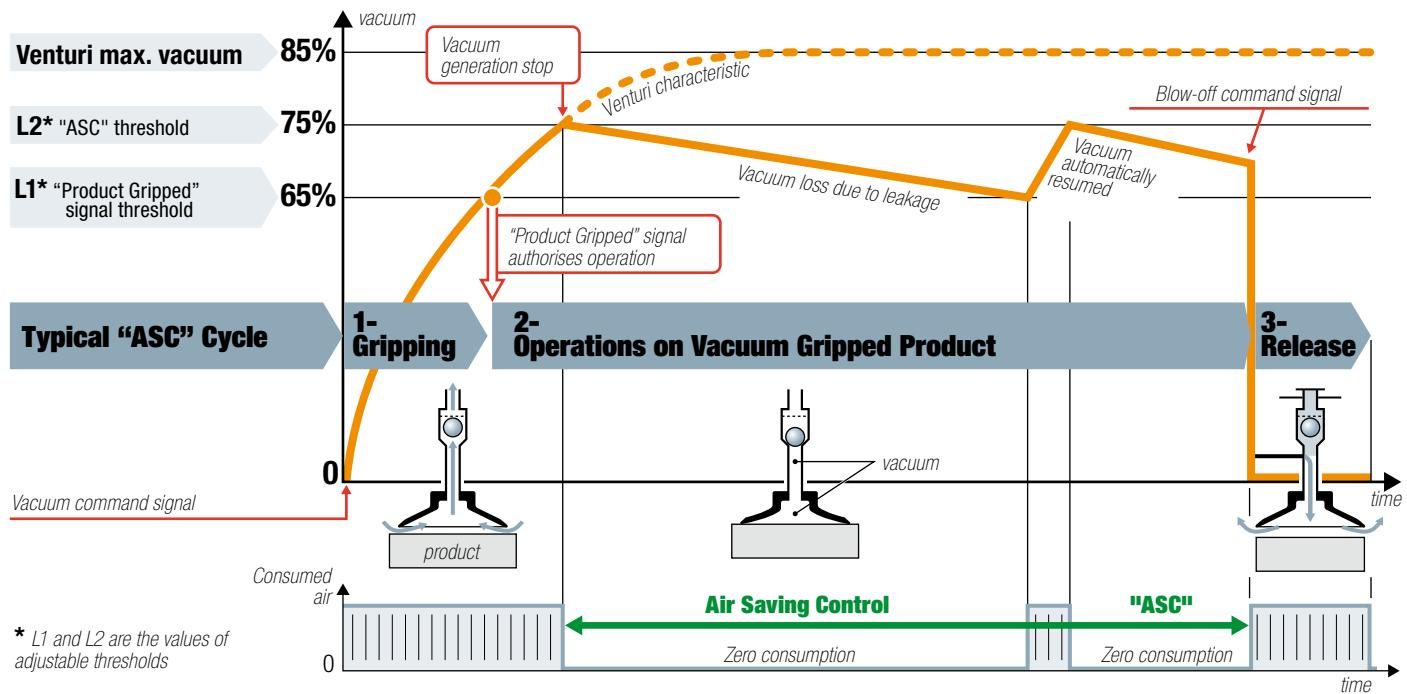
For airtight or semi-airtight products, the LEMAX+ pumps automatically run the above "ASC" cycle, thus resulting in maximum energy savings, according to the following three phases:
